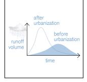
stormwater discharge before and after urbanization
