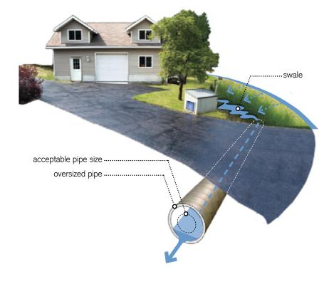
optimal level of service flow control
