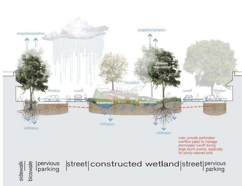
of stormwater runoff expected to enter the street. Stormwater runoff can also be harvested and stored underground for later use.
