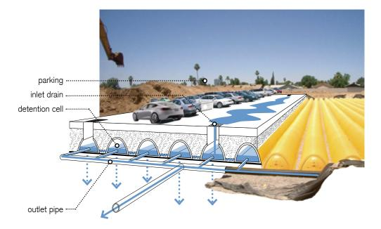
optimal level of service detention/infiltration
